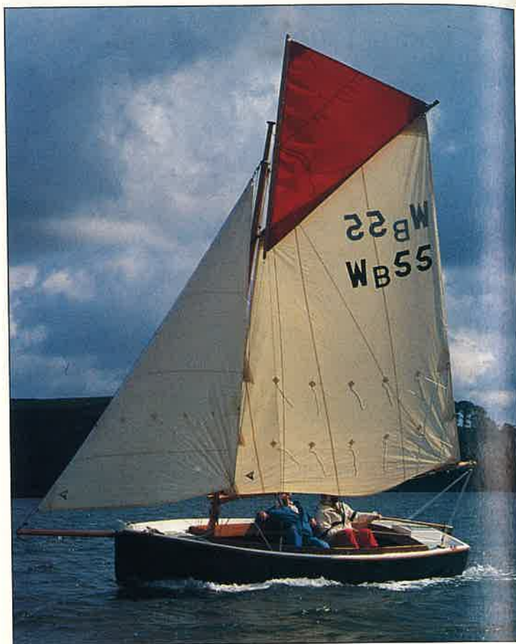
For the helmsman, the aft side benches are ideal for sitting with feet braced opposite, while for the crew the centre thwart and angled coaming allow for a relaxed, comfortable position with legs outstretched.
