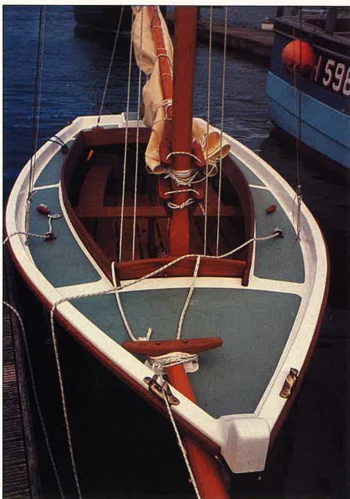
Top: Three-up: Eric moved to his favourite position out of the wind on the floorboards. Above: To house the offset bowsprit Eric cut through the bulwark and protected the hole with a specially fabricated inner moulding. The visible edges were then tidied up with a bronze trim and the removable bowsprit was installed.
